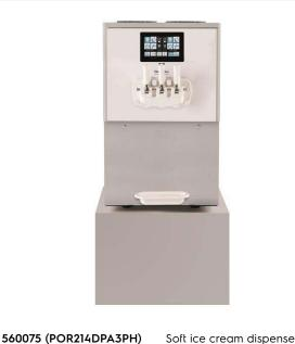
DR214DPA3PH) Soft ice cream dispenser with 2x8 I tank capacity and 1,95 I cylinder volume, 2 flavours + 1 mix, electronical control and touch screen panel, countertop, hourly production: 600 cones (75 gr), pump version, R452A
